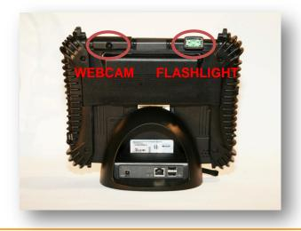
Additionally to this, the TRAVIS Mentor is ready to join videoconferences or remote-troubleshooting sessions. Therefore a webcam and a flashlight are integrated on the backside of the device. If you got stuck and need assistance, simply press a button on the Mentor and you will be directly connected to your Brückner service team via
